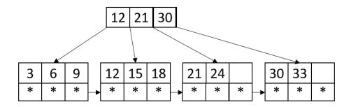
Here is a snapshot of a 2-4 B<sup>+</sup>-tree index, that is - each node in this B-tree must contain between 2 and 4 pointers.
